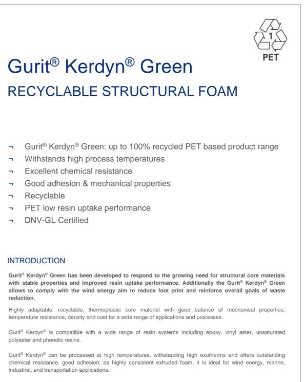
Applicable processing techniques include vacuum infusion, bonding, prepreg, and thermoforming. Available in a wide range of thicknesses.
